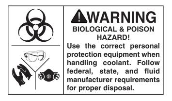
A small amount of coolant is lost during normal operation. Check the coolant tank regularly and fill it if necessary. We recommend changing the coolant every three months or sooner if it develops an unpleasant odor. However, be sure to follow the coolant manufacturer's instructions when checking, adding, or changing coolant.
